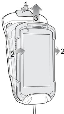
To ensure the device was inserted correctly, listen for the audible click that signifies that the device locking mechanism was enabled and the device was locked into place.
