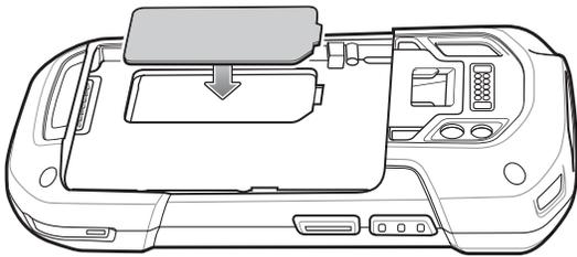
15. Press the access door down and ensure that it is properly seated.
