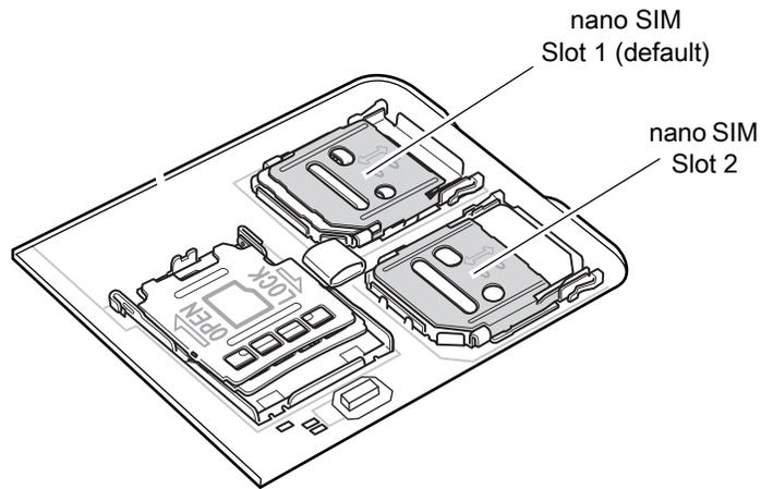
3. Slide the SIM card holder to the unlock position.
