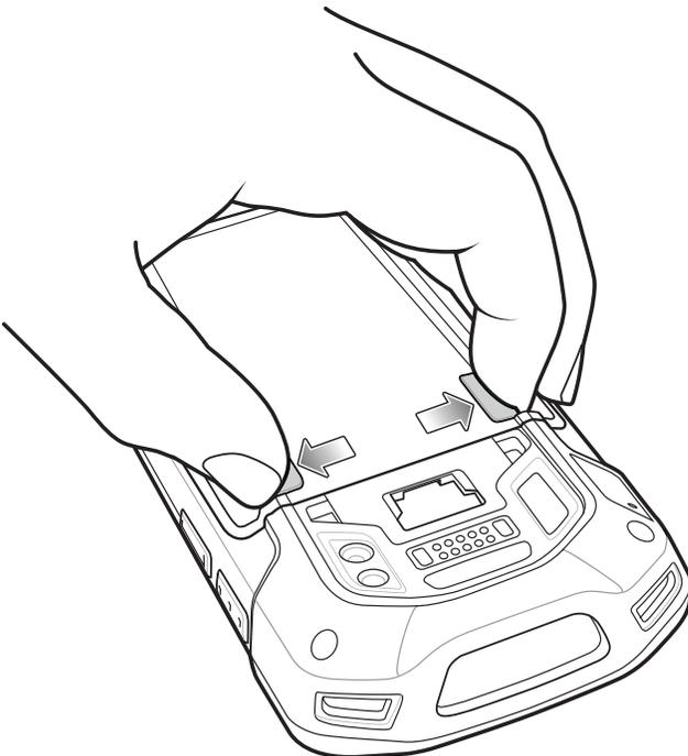
8. Lift the battery from the device.
