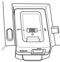
For Ethernet communication, slide the switch to the position.
