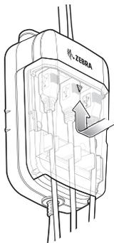
5. Slide cable cover up to lock into place.
