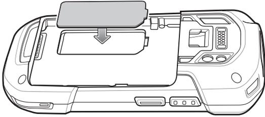
9. Press the access door down and ensure that it is properly seated.
