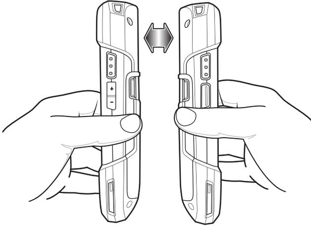
When the devices connect, a sound emits, the image on the screen reduces in size, the message **Touch to beam** displays.
