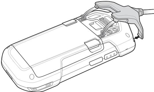
2. Rotate the cable down and press until it snaps into place. Magnetics hold the cable to the device.
