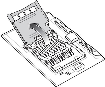
6. Insert the microSD card into the card holder door ensuring that the card slides into the holding tabs on each side of the door.
