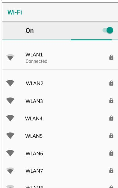
3. Scroll through the list and select the desired WLAN network.
