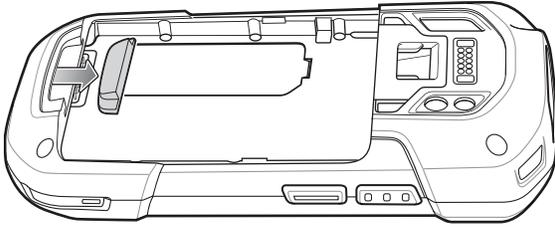
2. Insert the hand strap plate into the hand strap slot.
