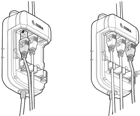
4. Align the cable cover onto the USB I/O Hub. Ensure that the cables are within the cover opening.
