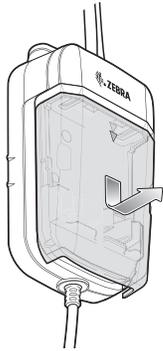
2. Insert the USB cable connector into one of the USB ports.
