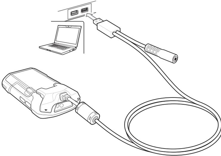
2. Connect the USB connector of the cable to a host computer.
