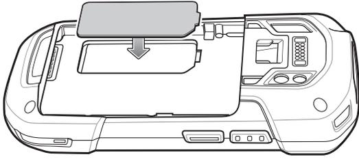
12. Press the access door down and ensure that it is properly seated.
