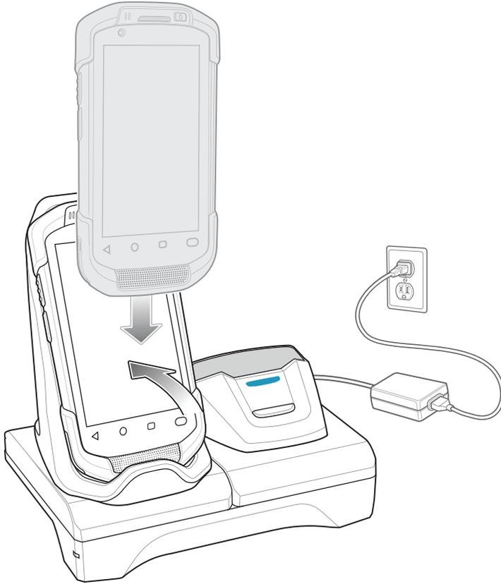
2. Rotate the top of the device until the connector on the back of the device mates with the connector on the cradle.
