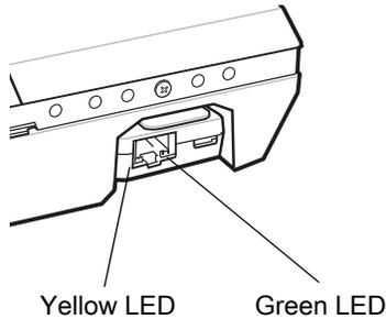
**Table 16** USB/Ethernet Module LED Data Rate Indicators
