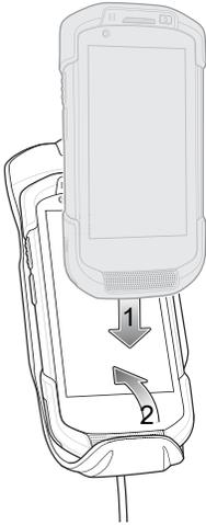
**Figure 192** Remove Device from Cradle
