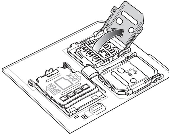
5. Place the nano SIM card into the card holder with contacts facing down.
