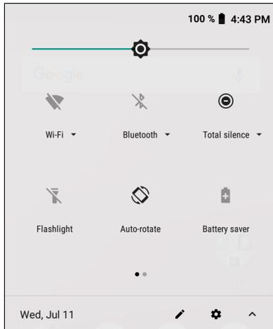
2. Touch **Wi-Fi** to open the **Wi-Fi** screen. The device searches for WLANs in the area and lists them.
