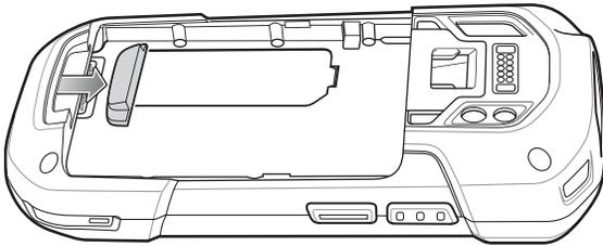
7. Insert the attachment plate into the hand strap slot.
