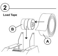
A: Slide tape roll onto core holder B: Place loaded core on holding bracket
