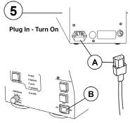
A: Connect power cord (in back) B: Press power switch (on front) to turn on the machine
