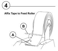
A: Affix tape onto feed roller B: Re-insert hold down shaft into guide.
