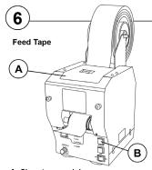
A: Close top panel door B: Press advance button to feed tape
