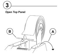
A: Open top door panel B: Remove hold down shaft guide from unit.
