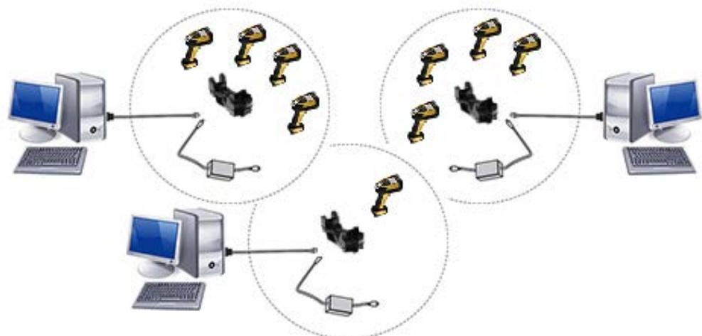
Many stand alone connections can operate in the same physical area without interference, provided all readers and base stations in the system have different addresses.
