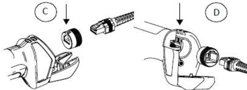
4. Once the cable is properly inserted, close the handle and screw it back into the body.
