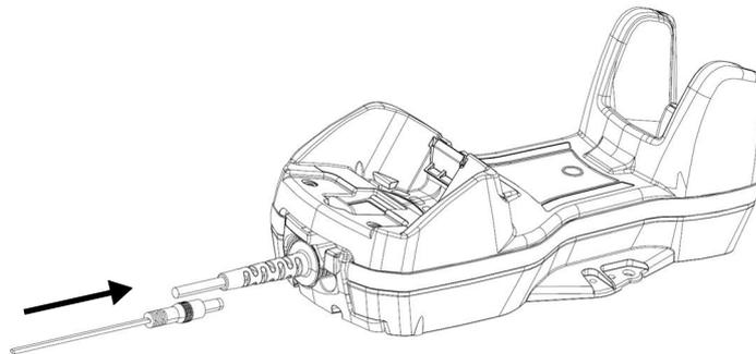
After connecting the power supply cable, secure it on the strain relief as shown in the figure below.
